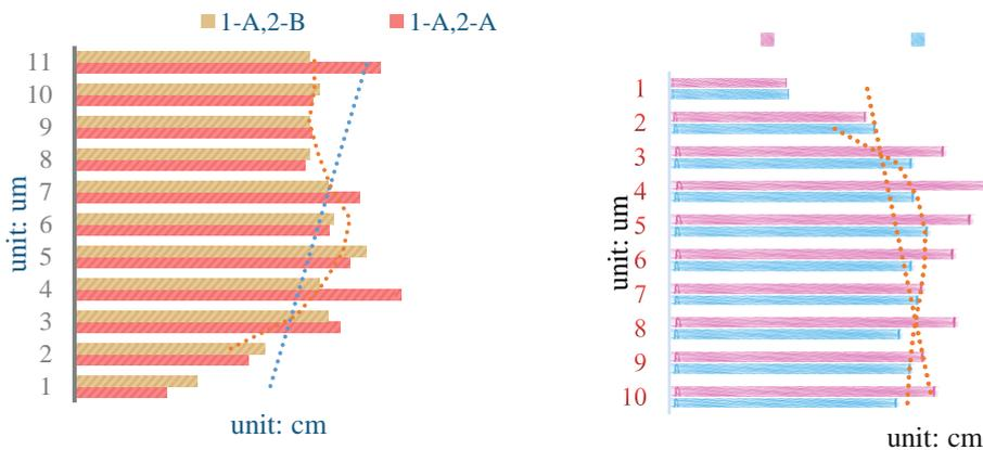
*Figure 7 Thickness of multi-atomized arc spray coating*
