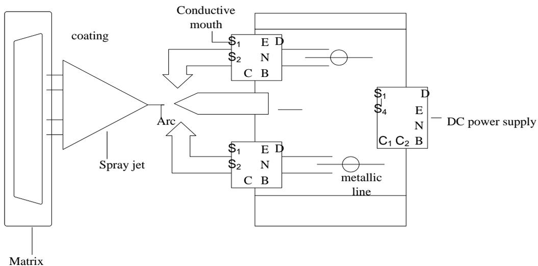
Figure 2 Schematic diagram of arc spraying principle
