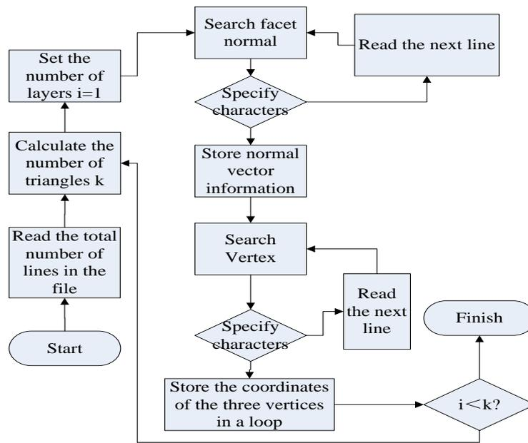
Figure 4 STL file reading algorithm flow chart
