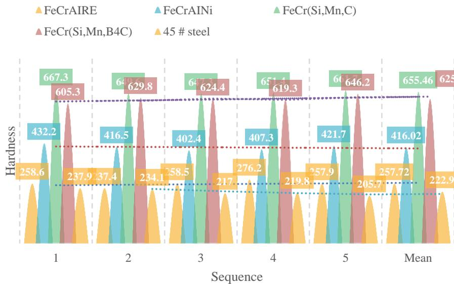
Figure 6 Hardness of arc sprayed nano-closed composite coating
