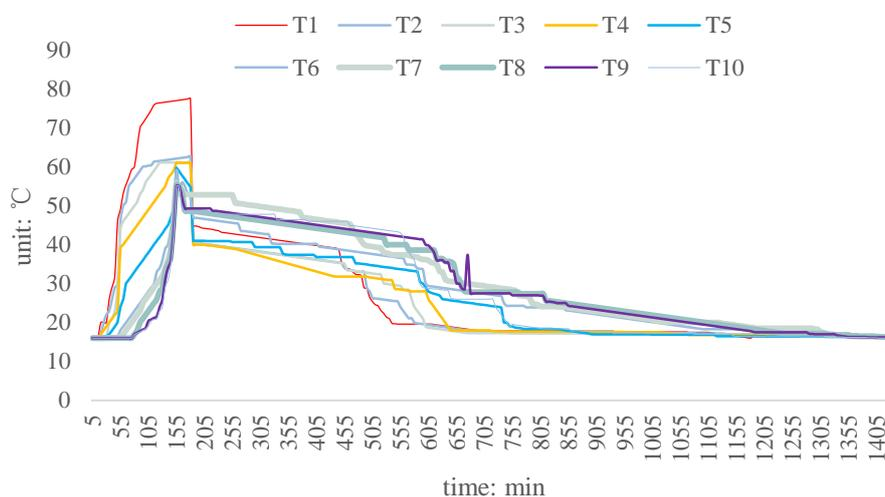
Figure 8 Temperature change curve of insulation board
