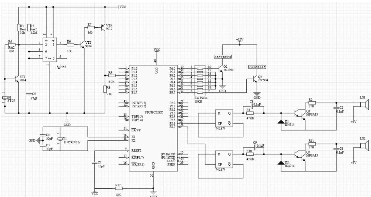
Figure 2: The schematic diagram of the connection of the microcontroller and modules.
