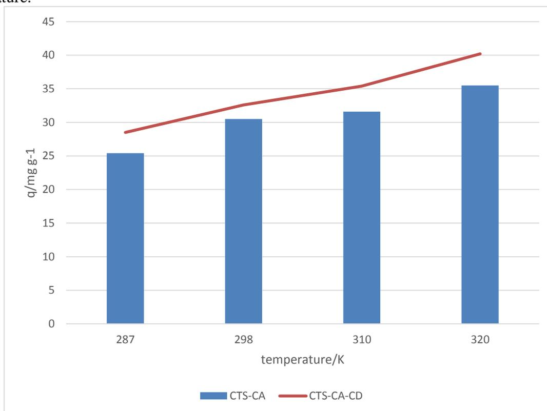
Figure 2. Effect of temperature on adsorption performance
