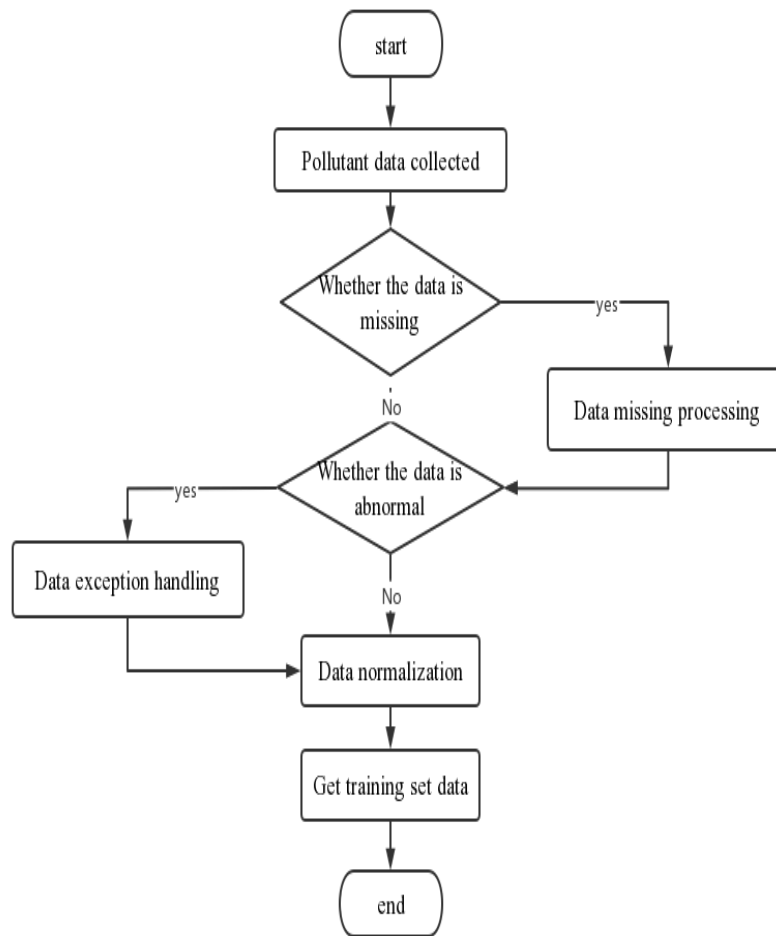
Figure 3. Flow chart of data preprocessing module
