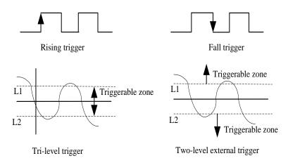
Figure 2. Diagram of trigger mode
