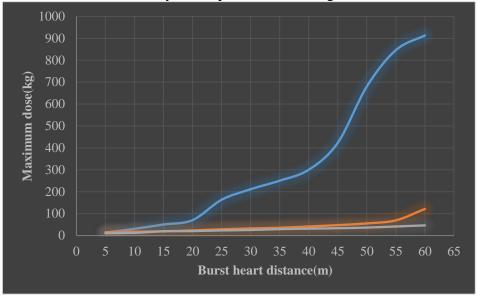
Figure 7. Relationship between the bursting heart distance and the maximum dose under the vibration speed allowed by the safety of adjacent buildings
