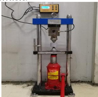
Fig .1 Point Load Test Equipment
