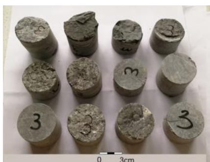
Fig.2 Point Load Test Specimen
