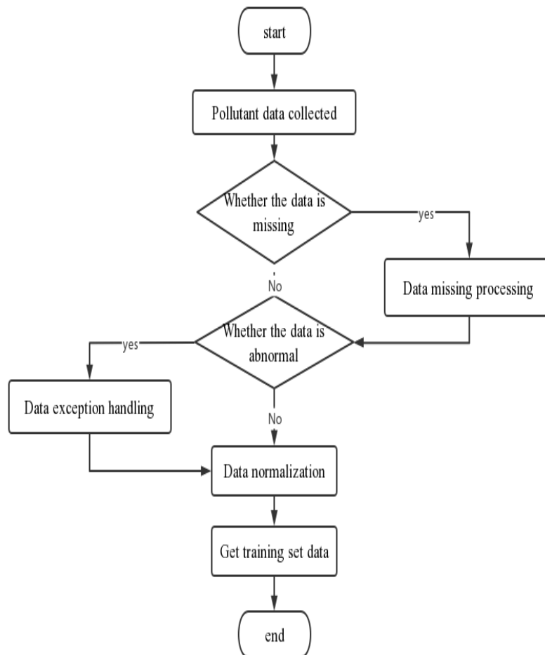
Figure 3. Flow chart of data preprocessing module
