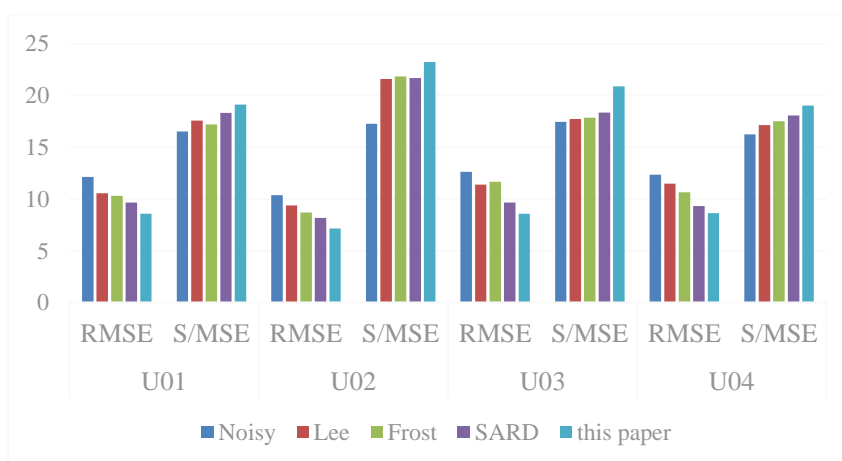
Figure 4. \sigma = 0.7 Histogram of values of RMSE and S/MSE of various denoising methods under speckle noise level
