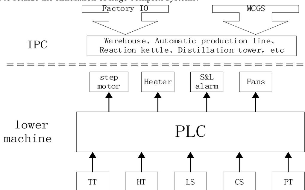
Fig 1. Operation diagram of typical industrial control objects
