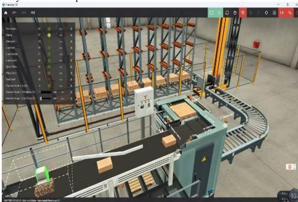
*Fig 3. Automated warehouse based on Factory IO*
