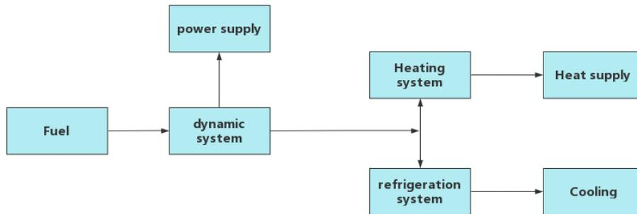
Figure 1. Energy supply process of CCHP system
