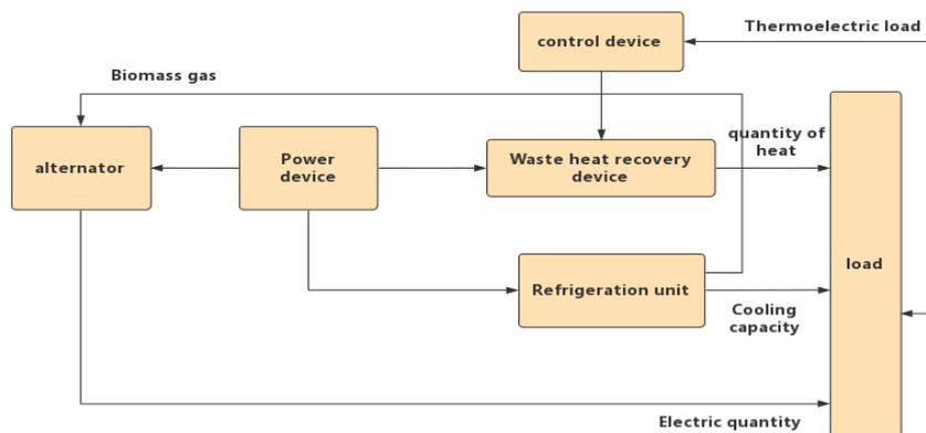
Figure 2. Schematic diagram of distributed biomass CCHP system
