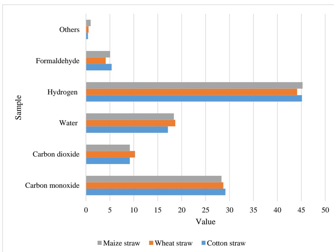
Figure 3. Syngas components generated from balanced solar-biomass gasification
