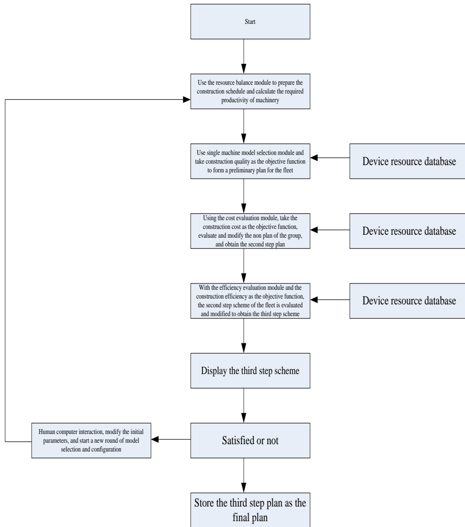
Figure 3. Resource balance optimization model of mechanical engineering project
