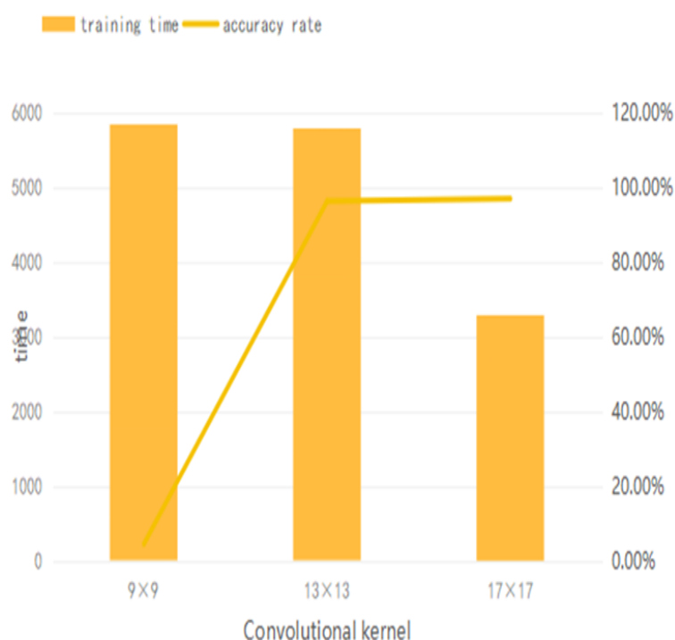
Figure 2. Effect of the size of the convolution kernel on the training time and accuracy
