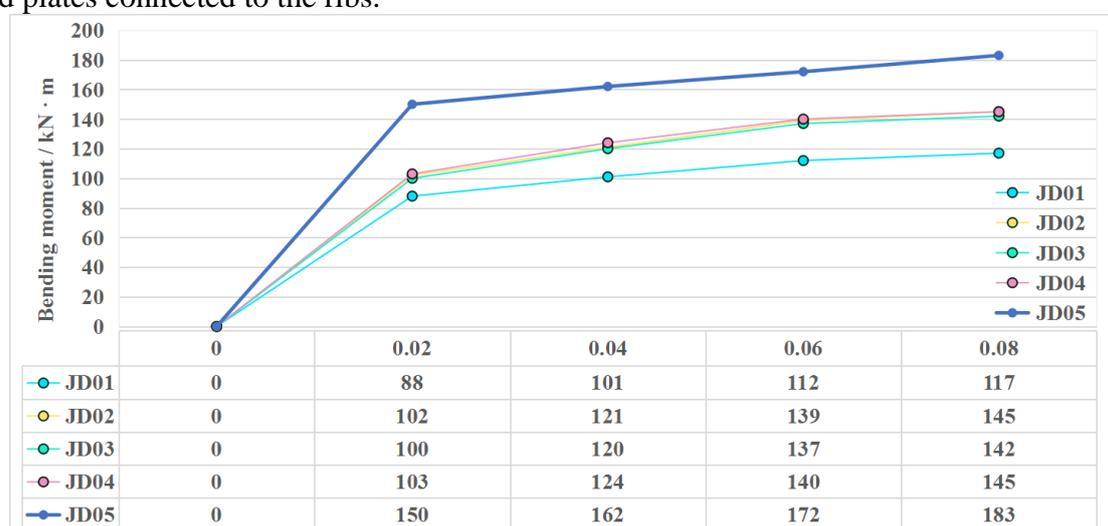
Figure 4. Relationship between bending moment and angle
