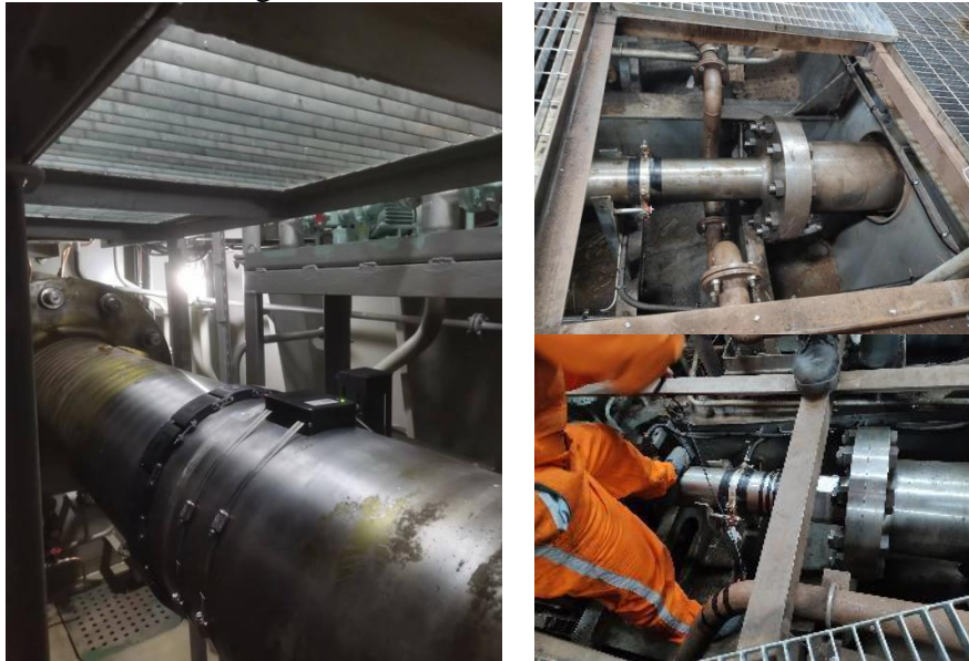
Figure 6. Shaft power meter installed in a 126m ship
