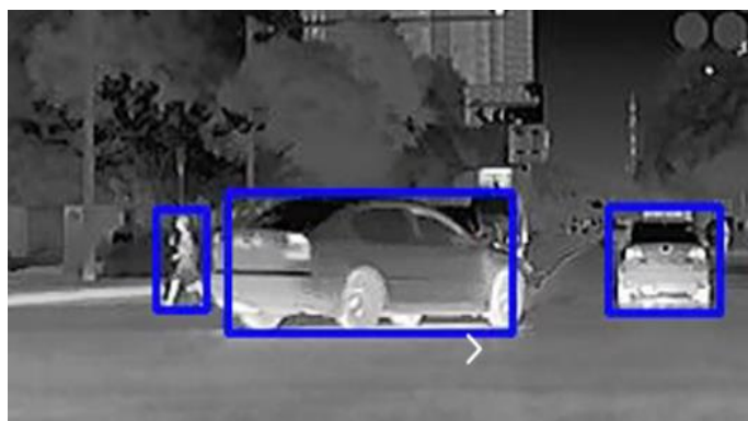
Figure 6. Infrared vehicle-mounted lens for vehicle recognition
