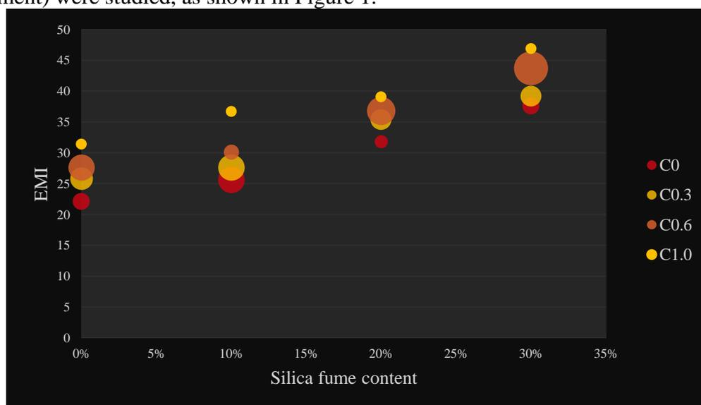
Figure 1. Shielding performance of electromagnetic wave
