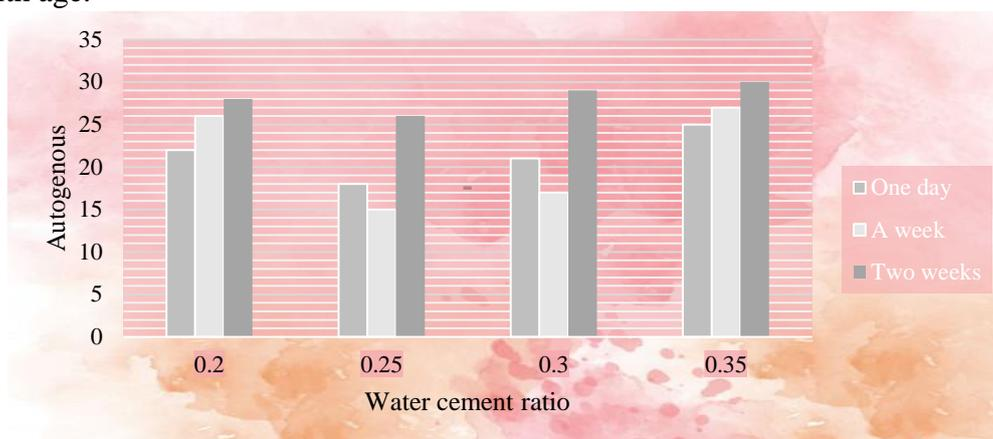
Figure 2. Autogenous shrinkage test of nano carbon fiber cement
