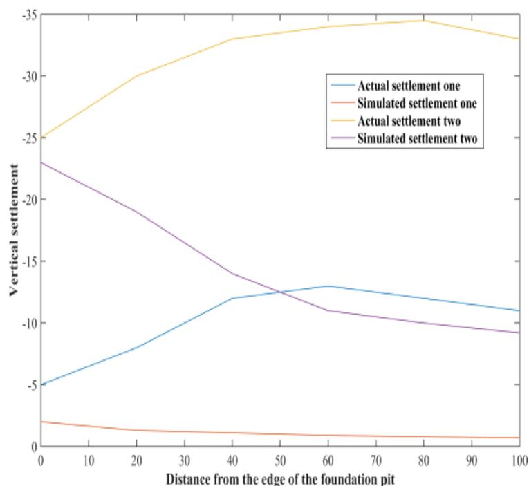
Figure 5. The actual value of precipitation excavation settlement and the second simulation line of working conditions
