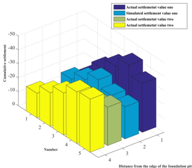
Figure 4. The actual value of precipitation excavation settlement and working conditions-a three-dimensional diagram of simulated values
