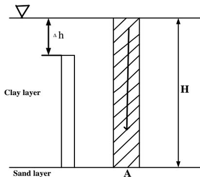
Figure 1. Schematic diagram of seepage
