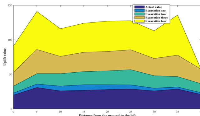
Figure 6. The area of the actual foundation pit bottom uplift value compared with the simulation value of the four excavations
