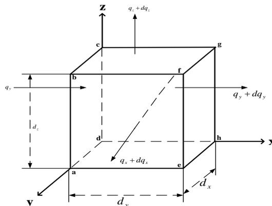
Figure 2. Schematic diagram of the unit in the seepage zone
