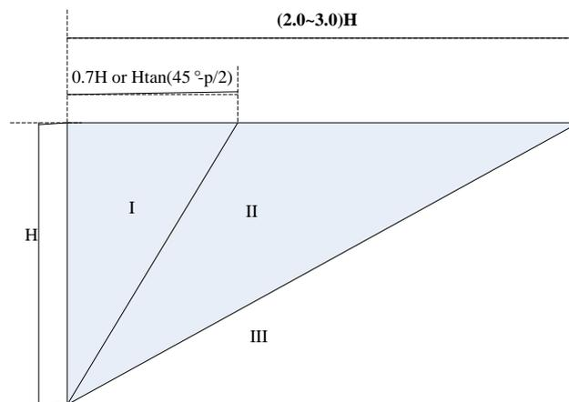
Figure 3. Impact zoning of foundation pit precipitation project
